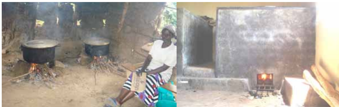
Figure 8.9: Cooking at Nyamnina Primary School using a three stone stove (left) and a fixed institutional Rocket stove (right)
