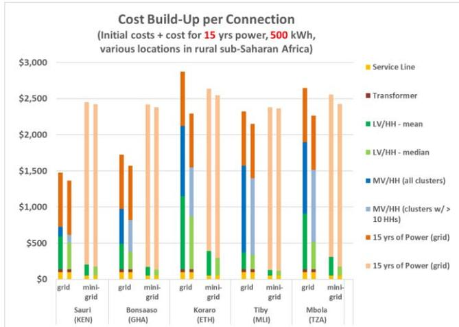
Figure 12: All costs – initial and recurring – estimated for grid and solar mini-grid electrification assuming 15 year duration and 500 kWh/HH-yr demand.
