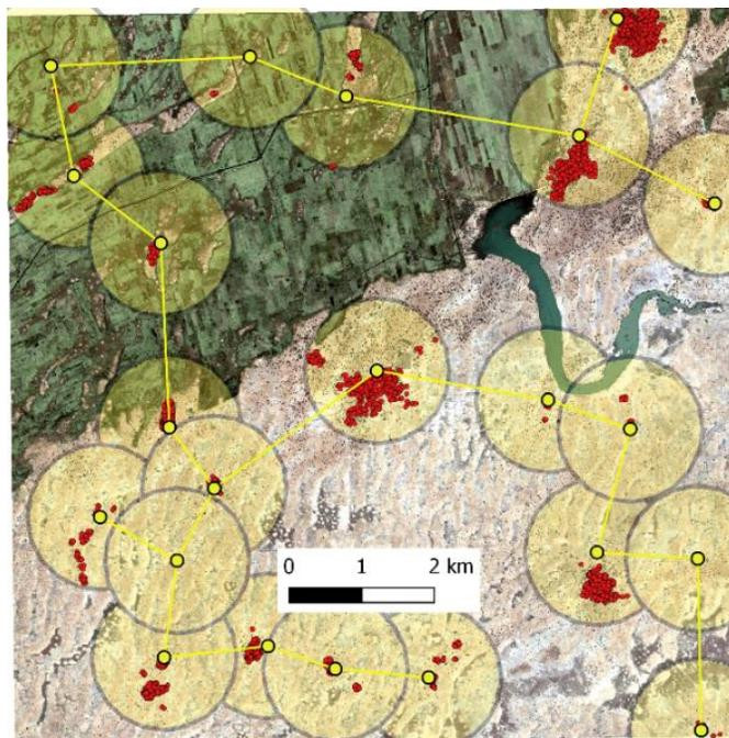
Figure 3: Rural Mali (Ségou Region, full Tiby village area, 10 km x 10 km): 2,496 rooftops (red points) identified in satellite imagery (~770 HHs) in 22 clusters with 1000 m radius (yellow points and circles) connected by ~37 km MST (yellow line).
