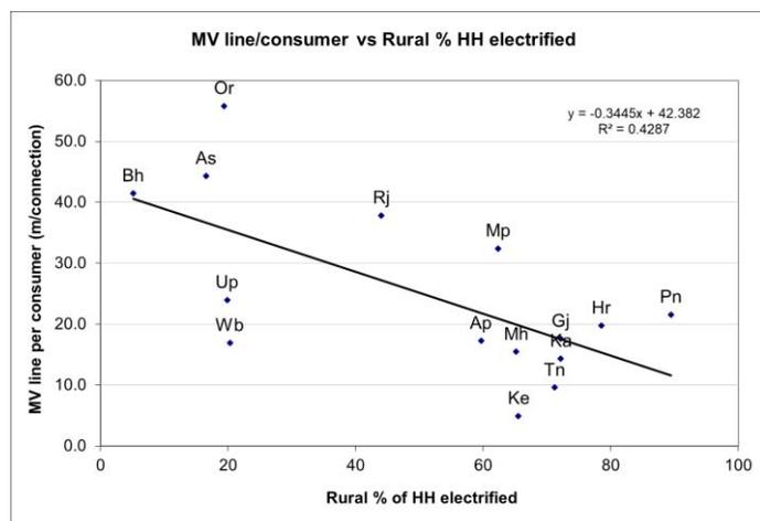
**Figure 18: Rural electrification rates versus MV line length for states in India.**
