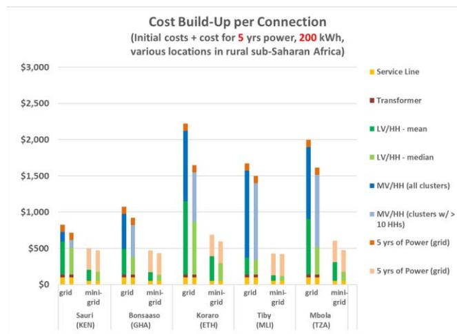
**Figure 11: All costs – initial and recurring – estimated for grid and solar mini-grid electrification assuming 5 year duration and 200 kWh/HH-yr demand.**
