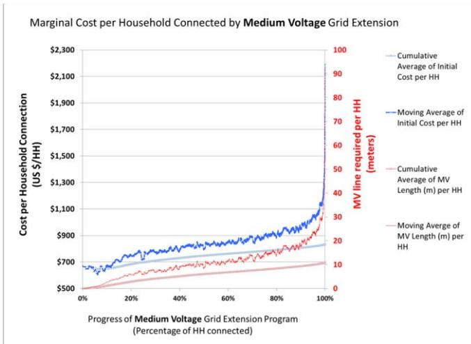
Figure 14: Increasing MV line and cost as prioritized grid roll-out proceeds (northern Nigeria)
