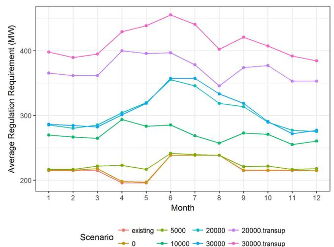
Fig. 7. Monthly computed average regulation requirements. (Note: The “existing” regulation requirements can be difficult to see because, aside from some slight variation in Months 3–4, they align with the 0 GW wind power capacity simulation.)
