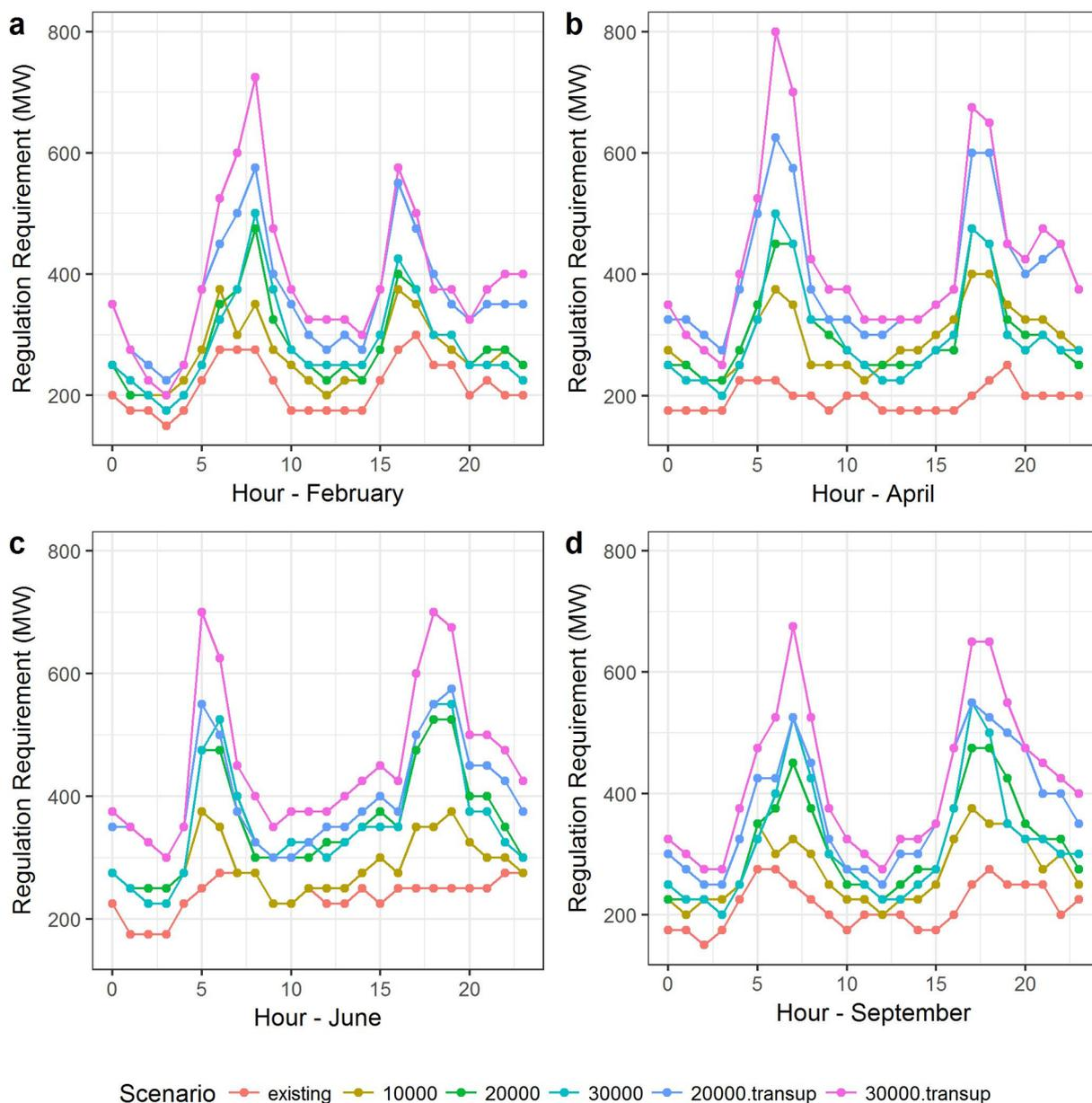
Fig. 8. Hourly computed regulation requirements for representative months and select simulated wind power capacities.
