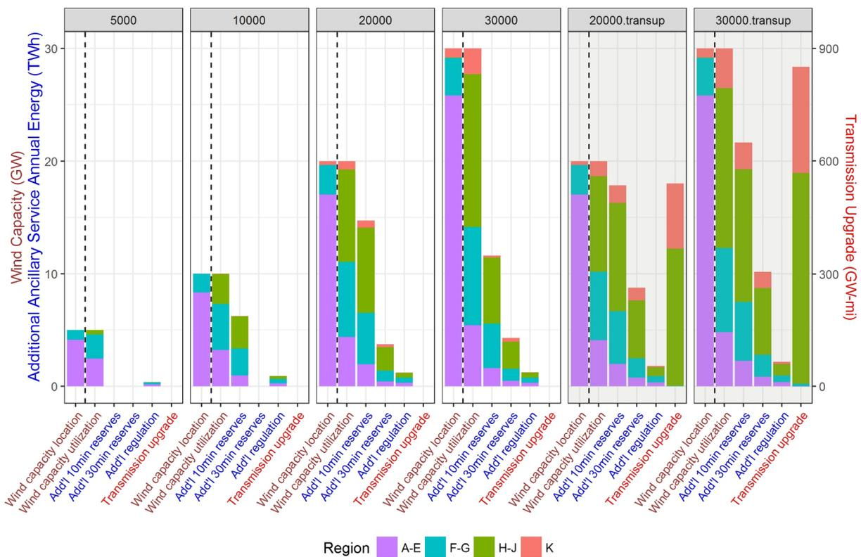
Fig. 11. Distribution of investments in and utilization of energy infrastructure with increasing wind power and transmission capacities. Note: horizontal axis text color corresponds to text color for corresponding vertical axis parameter.
