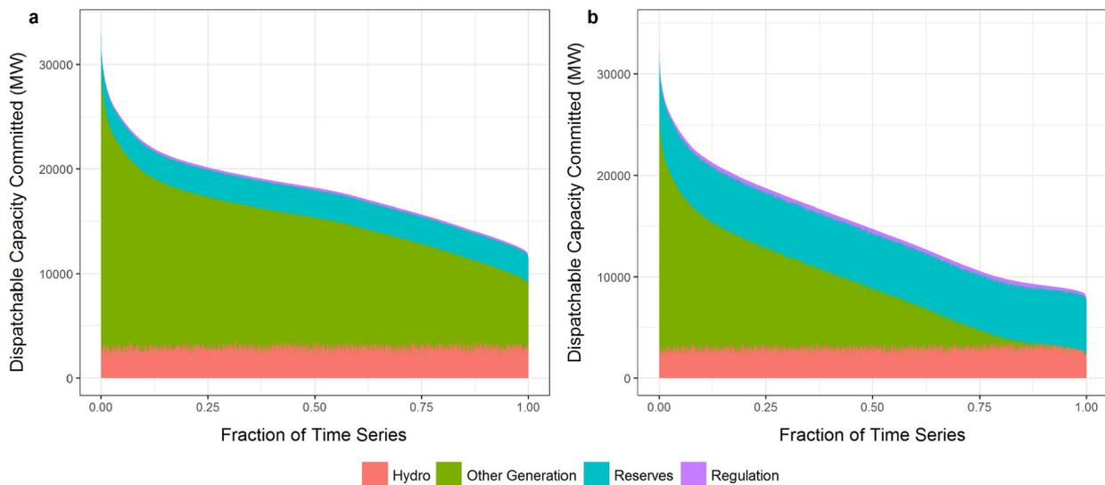
**Fig. 10.** Distribution of total dispatchable capacity committed to energy services (i.e. “Hydro” and “Other Generation”) and ancillary services (“Reserves” and “Regulation”) over the full simulation time series: (a) No new wind power scenario; (b) 30 GW wind power with upgraded transmission scenario.
