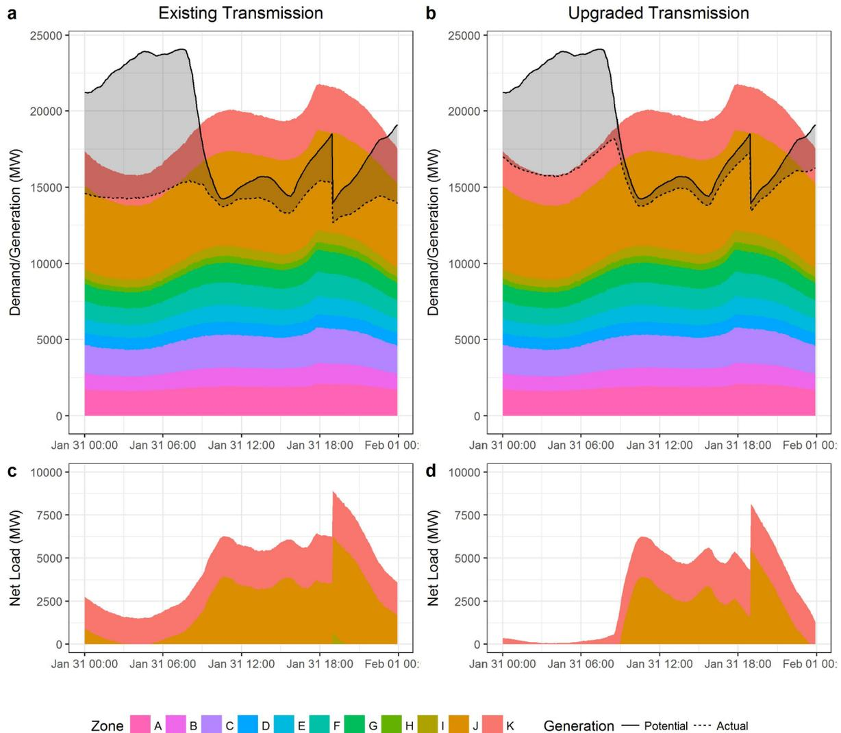
**Fig. 5.** Time series, with five-minute time steps, of simulated day with largest net load ramp in 30 GW wind power scenarios: (a) Zonal electricity demands (stacked areas), total statewide potential and actual low-carbon electricity for existing transmission constraint scenario; (b) analogous to (a) with upgraded transmission limits; (c) zonal net load corresponding to (a); and (d) zonal net load corresponding to (b).
