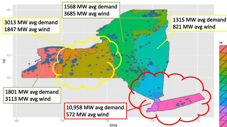
Fig. 1. NYISO zones [37] and distribution of average electricity demand [37] and average potential wind power [13]; both correspond to the years 2007–2012. Wind values correspond to average output in the full 37.8 GW capacity data set at wind sites indicated by points [40].
