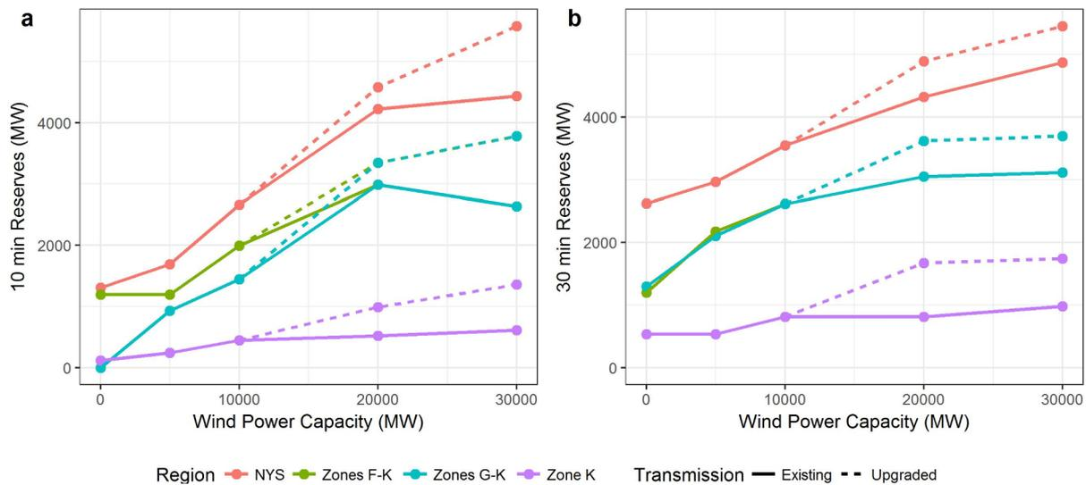
**Fig. 9.** Regional operating reserve requirements with increasing wind power capacities with existing and upgraded transmission limits: (a) 10-min total reserves and (b) 30-min total reserves. Note: The existing Zone K 30-min reserve requirement varies by hour; for simplicity here, only the peak existing 540 MW is shown.
