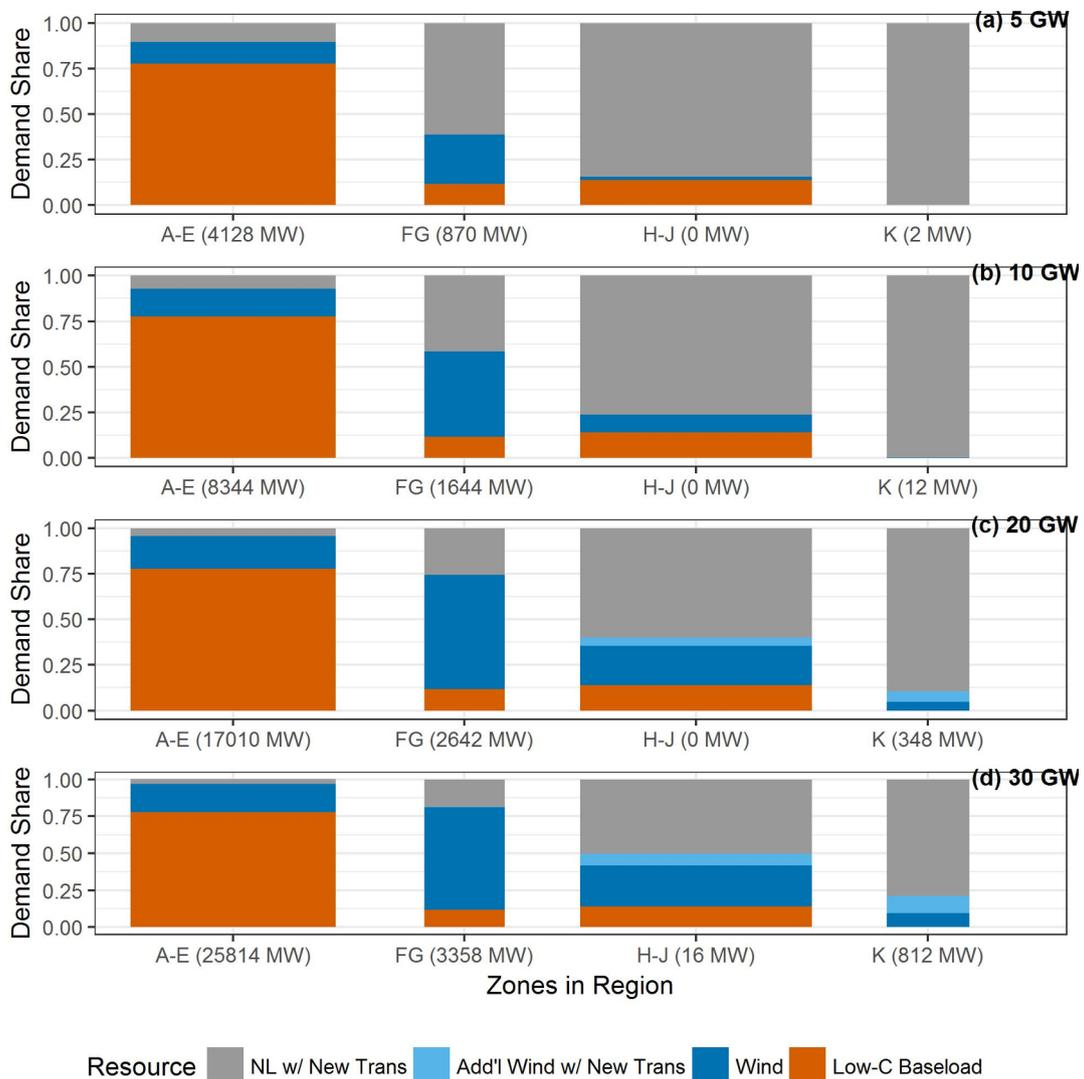
Fig. 3. Simulated share of total six-year demand met by low-carbon generation in select regions for statewide wind power capacity scenarios of (a) 5 GW, (b) 10 GW, (c) 20 GW and (d) 30 GW. The width of each bar is scaled to the average demand: Zones A–E 6383 MW, Zones F–G 2495 MW, Zones H–J 7211 MW and Zone K 2567 MW.
