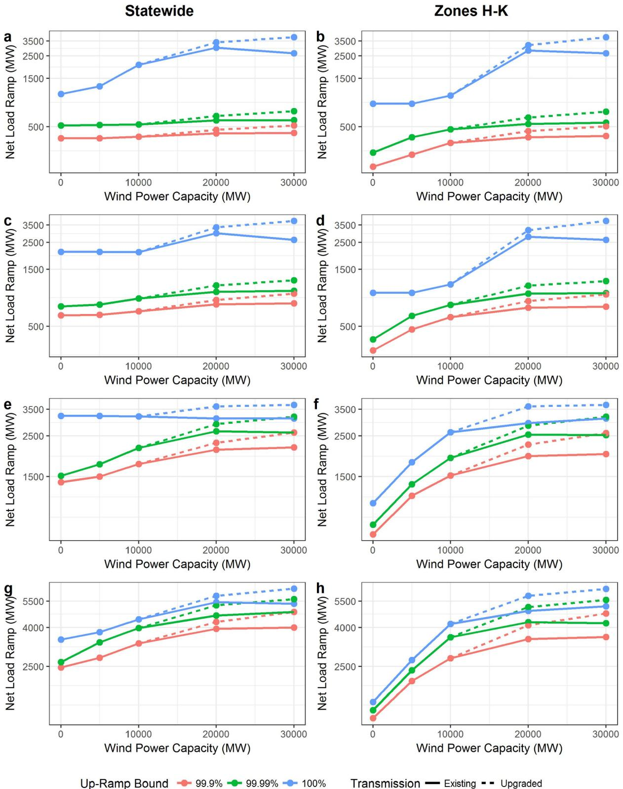
Fig. 6. Extreme net load up-ramps Statewide and in Zones H-K over the six-year analysis period: (a) Statewide 5-min NLR, (b) Zones H-K 5-min NLR, (c) Statewide 10-min NLR, (d) Zones H-K 10-min NLR, (e) Statewide 30-min NLR, (f) Zones H-K 30-min NLR, (g) Statewide one-hour NLR, (h) Zones H-K one-hour NLR.
