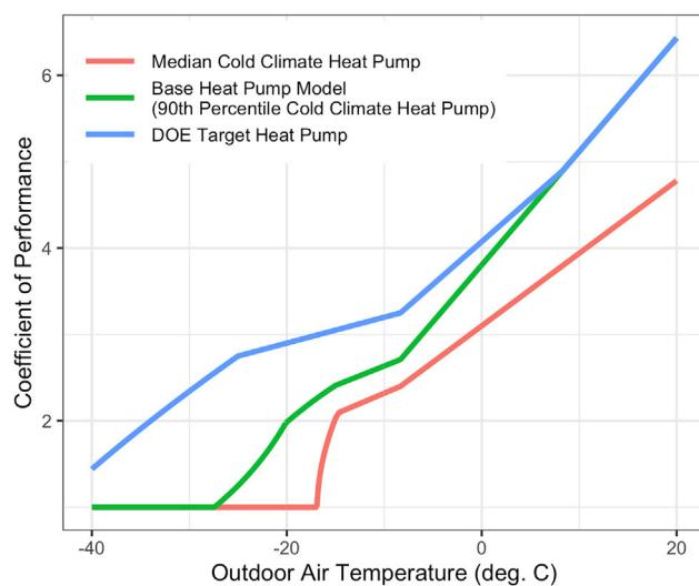
Figure 8. Heat Pump Model Temperature-Dependent Coefficient of Performance
