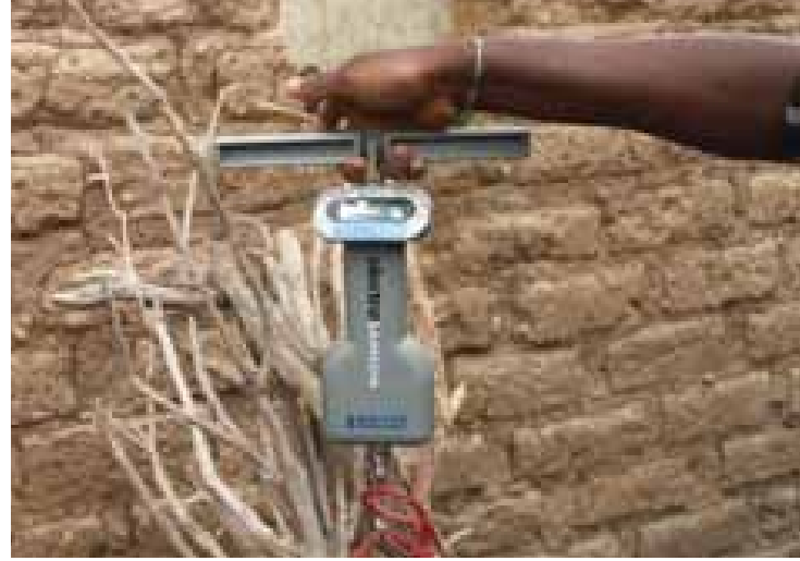
Figure 4.9: CCTs: Simultaneous Cooking Tests on Multiple Stoves (left); Weighing Fuelwood Consumed (right)
