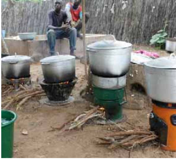
Figure 4.9: CCTs: Simultaneous Cooking Tests on Multiple Stoves (left); Weighing Fuelwood Consumed (right)
