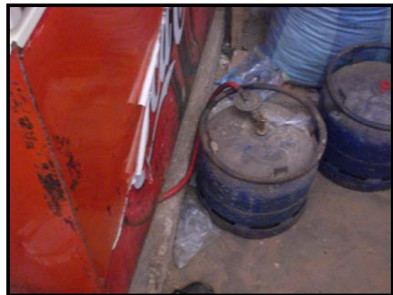
Picture 46: Refrigerator that runs on LPG
