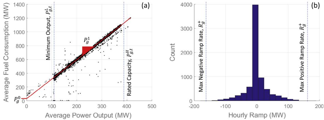
**Fig. 3.** Description of generator data and derivations of performance parameters for fossil fuel generators. Generator rated capacity: 387 MW, steam turbine fueled by natural gas. (a) Plot of the hourly fuel consumption and power output as reported in the RGGI. Parameters shown for maximum rated capacity, minimum output, and linear heat rate. (b) Histogram of the hourly change in output (excluding changes to 0 MW). Parameters for maximum negative and positive ramp rates shown.
