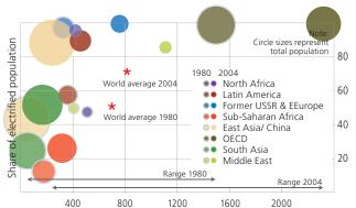
Mean residential electricity consumption per electrified inhabitant in kWh
