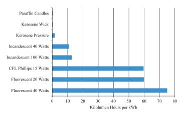
Figure 19.10 | Relative efficiency of different sources of lighting. Source: World Bank, 2010b.
