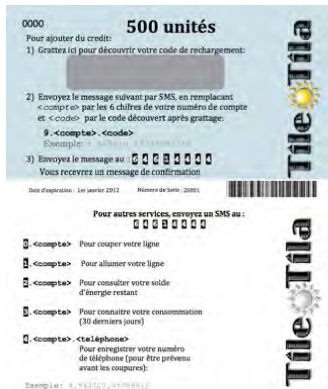
Figure 6: Scratch cards for electricity purchase. Cards contain a concealed authorization code as well as instructions on how to add credit to the customer account and how to get account information.
